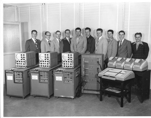
Image 1: Development team with three MADDIDA machines of Northrop Aircraft 1949. „The advances in MADDIDA in terms of simplicity and miniaturization are of great significance to the scientific and business world. A desk-side mechanical brain.“ Press release. (Computer Museum Mountain View, document no. 10885, 102710219)
