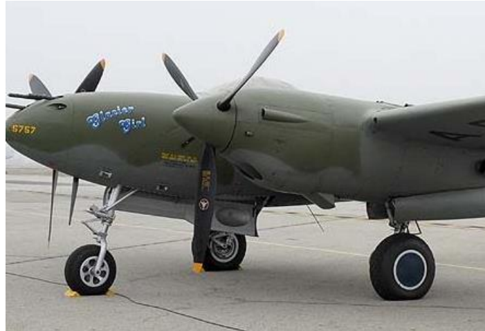
Image 3: Landing Gear of Lockheed P38 (Image Press Release)
